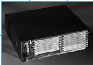
Cable Modem Redundant Switches
